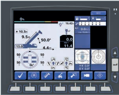
Startup screen of crane control AML-F
